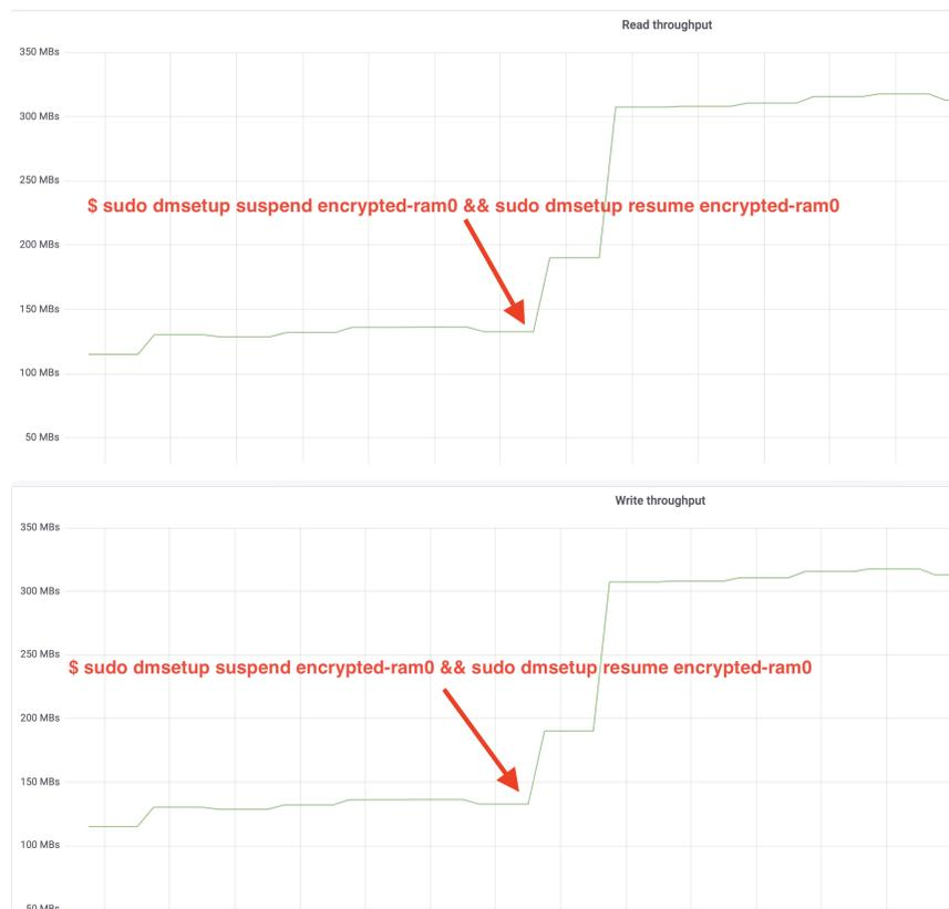
Wow, we have more than doubled the throughput! With the total throughput of  $\sim 640$  MB/s we're now much closer to the expected  $\sim 696$  MB/s from above. What about the IO latency? (The `await` statistic from the [iostat reporting tool](#)):
